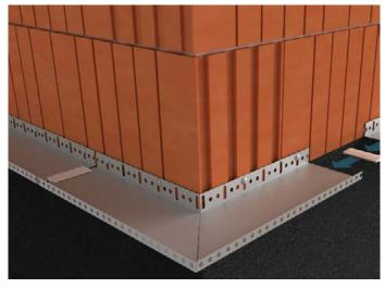
The SOLTHERM STARTER TRACK is installed at DPC level and at least 150 mm above ground. The starter track is mechanically fixed at 300 mm centres with specified fixing and approx. 50 mm from the edge.
