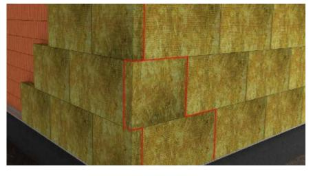
External corners are formed as per a brickwork corner, ensuring a full brickbond.
