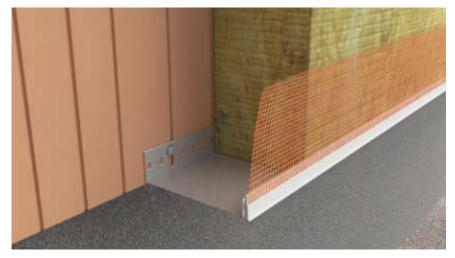
The first course of dual density mineral wool boards are placed into the SOLTHERM STARTER TRACK with the mesh of the clip on bead facing outwards.
