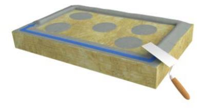
Once the contact layer is applied, apply further insulation adhesive to the perimeter and where the dabs are located.
