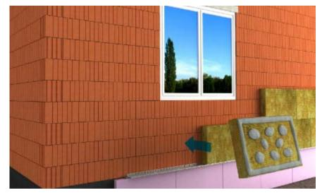
Insulation boards must be placed against the substrate in a brickbond manner achieving a minimum 150mm stagger with the above/below insulation panel.
