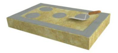
Repeat the contact layer application for 6-8 large dabs (80-100mm) to the centre of the board.
