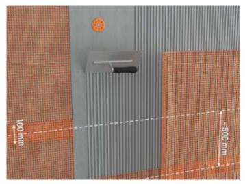
All secondary reinforcing mesh must maintain a minimum overlap of 100 mm with adjacent mesh and all mesh joints must be staggered approximately 500 mm from the joints the first reinforcing mesh application.
