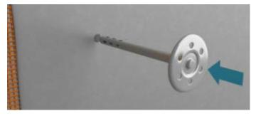
Drill an 8 mm diameter hole through the scrim and wet base coat at the required depth. Insert the stainless steel fixing into the hole with your hand as far as physically possible
