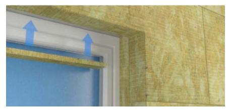
If windows are flush with the substrate, the main elevation insulation panels can simply over sail onto the window frame a minimum 20mm.
