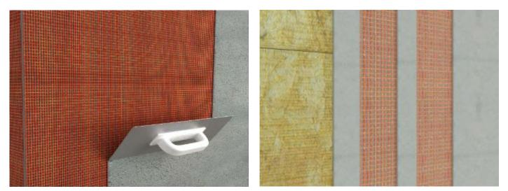
Allow the base coat to dry for approximately 24 hours before applying a tight slurry coat 1-2mm if required. The overall thickness of the base coat for ULTIMATE HD SILICONE & ULTIMATE HD ACRYLIC system should be between 4-6mm with two reinforcing meshes.
