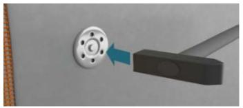
Using a hammer, gently hit the fixing centrally until it is recessed within the mesh and base coat approx. 1-2mm. While the base coat is still wet for ULTIMATE SILICONE & ULTIMATE ACRYLIC, placea mesh patch (100x100mm) over the fixing head and smooth over with additional base coat if required.
