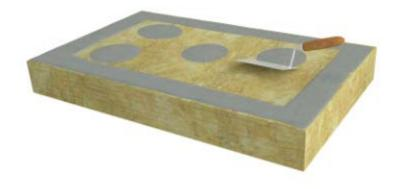
Repeat the contact layer application for 6-8 large dabs (80-100mm) to the centre of the board.
