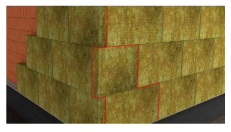
External corners are formed as per a brickwork corner, ensuring a full brickbond.
