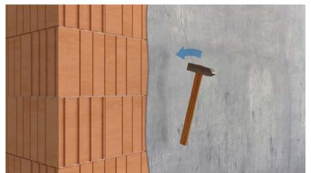
All heavy fungal growth must be removed from the substrate by either scraping or power wash and allowed to dry.
