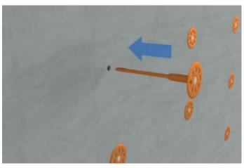
Place the fixing into the pre-drilled hole and push the fixing in until the head of the fixing is flush with the face of the base coat.
