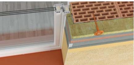
If windows are flush with the substrate, the main elevation insulation panels can simply over sail onto the window frame a minimum 20 mm.
