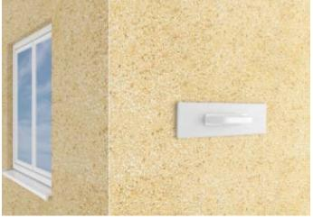
For plain opening, reveals/ingoes & heads, it is recommended SOLTHERM SDR is applied over 2 passes 'wet on wet' to an even thickness of 6-10mm. Once SOLTHERM SDR has sufficiently cured, a sponge float can be used to remove trowel lines and achieve a smooth and consistent finish. If required, apply SOLTHERM SNP & SOLTHERM STC-P Silicone Paint as per project specification.
