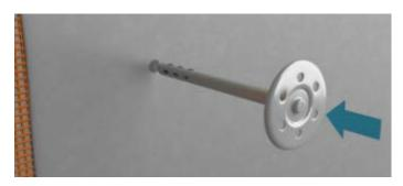
Drill an 8 mm diameter hole through the scrim and wet base coat at the required depth. Insert the stainless steel fixing into the hole with your hand as far as physically possible.
