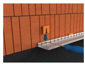
If the substrate is undulating and not line and level, it is acceptable to use packers.
