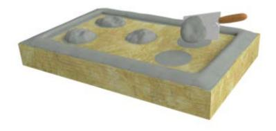
The adhesive thickness of the insulation adhesive layer, after pressing against the substrate wall, must be  $\leq 10$  mm and cover  $\geq 40\%$  of the overall area of the board.
