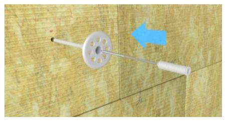
Place the fixing into the pre-drilled hole and push the fixing in until the head of the fixing is flush with the face of the insulation.
