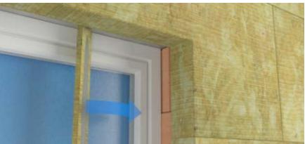
Where windows have recessed reveals and or heads, oversail the insulation board beyond the existing to create a channel to set a 30 mm thick mineral wool insulation strip in place within the reveal, adhesively fit as appropriate.
