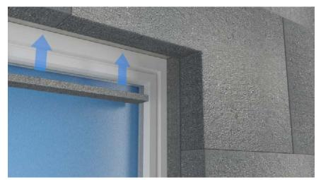
Where windows have recessed reveals and/or heads, oversail the insulation board beyond the existing to create a channel to set 20 mm or 30 mm thick EPS insulation strip in place within the reveal, adhesively fit as appropriate.
