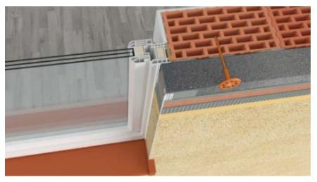
Ilf windows are flush with the substrate, the main elevation insulation panels can simply over sail onto the window frame a minimum 20 mm.
