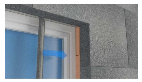
Alternatively, insulation at recessed reveals and/or heads can be mechanically fixed. Fixing are installed through the insulation at maximum 300 mm centres.
