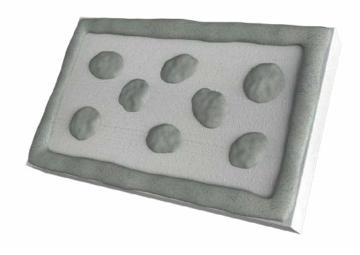
The adhesive thickness of the insulation adhesive layer, after pressing against the substrate wall, must be  $\leq 10$  mm and cover  $\geq 40\%$  of the overall area of the board.
