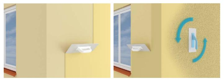
The silicone-acrylic texture coat SOLTHERM AF-P+ 15 or silicone texture coat SOLTHERM SFC-P 15 is applied to the required thicknesses (1.5 mm grain size), using a stainless steel trowel and finished with a plastic float to create a textured finish. The drying time is dependent on weather conditions.
