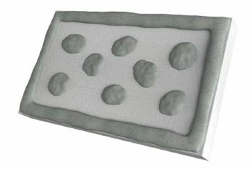
The adhesive thickness of the insulation adhesive layer, after pressing against the substrate wall, must be  $\leq 10$  mm and cover  $\geq 60\%$  of the overall area of the board.
