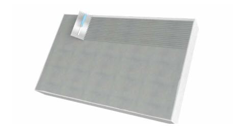
The insulation board is then pressed against the substrate wall and should achieve  $\geq 90\%$  contact area.
