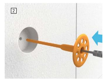
In the pre-drilled and cleaned hole place the fixing and push the fixing in until the head of the fixing is flush with the face of the pre-drilled gap.
