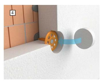
Install the anti cold-bridge EPS cap.
