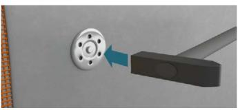
Using a hammer, gently hit the fixing centrally until it is recessed within the mesh and basecoat approx. 1-2 mm. Whilst the base coat is still wet, place a mesh patch (100x100 mm) over the fixing head and smooth with additional base coat if required.
