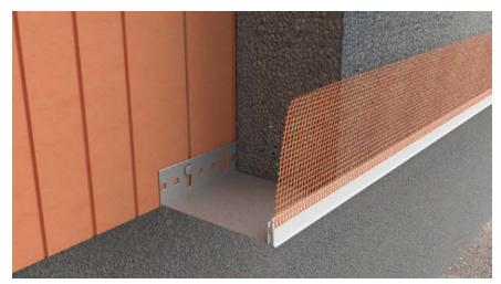
The first course of Grey EPS boards are placed into the SOLTHERM STARTER TRACK with the mesh of the clip on bead facing outwards.
