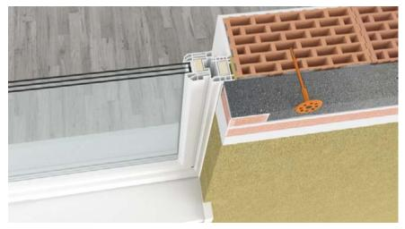
If windows are flush with the substrate, the main elevation insulation panels can simply over sail onto the window frame a minimum 20 mm.
