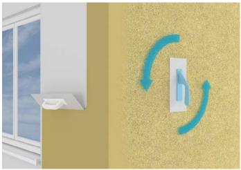
The silicone-acrylic texture coat SOLTHERM AF-P+ 15 or silicone texture coat SOLTHERM SFC-P 15 is applied to the required thicknesses (1.5 mm grain size), using a stainless steel trowel and finished with a plastic float to create a textured finish. The drying time is dependent on weather conditions.
