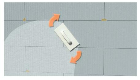
Where approved by the ICF system manufacturer, it is recommended that the outer surfaces of the EPS insulation panels, are lightly rasped with coarse sandpaper or an abrasive float rasp for EPS, to remove dust from the EPS surfaces.
