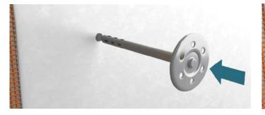
Drill an 8 mm diameter hole through the scrim and wet base coat at the required depth. Insert the stainless steel fixing into the hole with your hand as far as physically possible.
