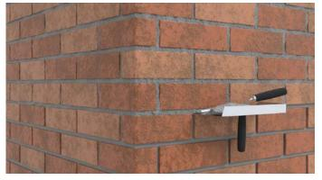
Place the fixing into the pre-drilled hole and push the fixing in until the head of the fixing is flush with the face of the base coat.
