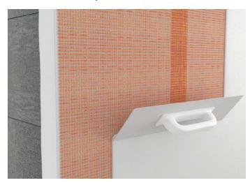
Allow the basecoat to dry for approximately 24 hours before applying a tight slurry coat 1-2 mm. The overall thickness of the basecoat should be relatively thicker between 4-6mm.
