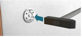
Using a hammer, gently hit the fixing centrally until it is recessed within the mesh and base coat approx. 1-2mm.
