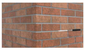
Screw or hammer the fixing into place ensuring the central pin is either flush with the fixing head or slightly recessed. The fixing head should be slightly recessed into the scrim coat face about 1-2mm.
