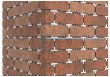
Following the general practices of brick laying, paying particular attention to the brick bond, apply the remaining brick slips, using plastic packers as guides to maintain the required joint width. Laser levels and string lines should be used to ensure application of the slips is level.
