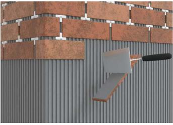
Apply a light contact layer of SOLTHERM SE to back of the individual brick slips. Always ensure full coverage.
