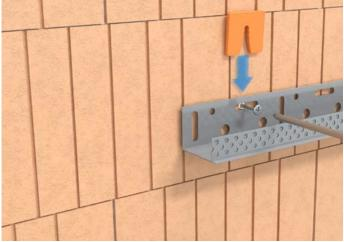
If the substrate is undulating and not line and level, it is acceptable to use packers.
