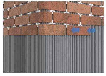
Firmly press the brick slip into place using a horizontal pushing motion, ensuring the collapse of the notched adhesive and 100% adhesion.
