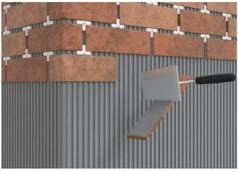
Apply a light contact layer of SOLTHERM E or SOLTHERM SE to back of the individual brick slips. Always ensure full coverage.
