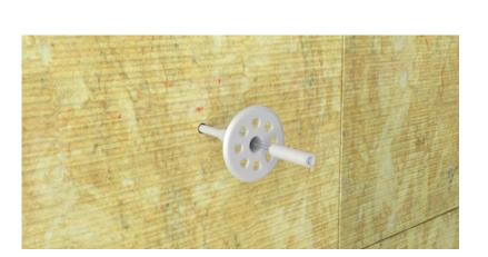
Screw or hammer (depending on fixing specification) the fixing into place ensuring the central pin is either flush with the fixing head or slightly recessed. The fixing head should be slightly recessed into the insulation face about 1-2mm.
