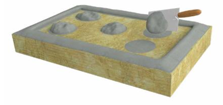
The adhesive thickness of the insulation adhesive layer, after pressing against the substrate wall, must be  $\leq 10$ mm and cover  $\geq 60\%$  of the overall area of the board.
