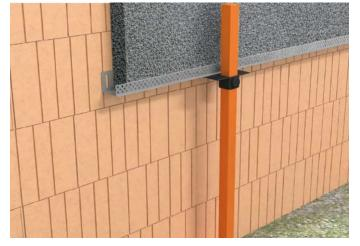
Due to the weight of the EPS insulation, it may be a requirement to temporarily support the SOLTHERM STARTER TRACK.
