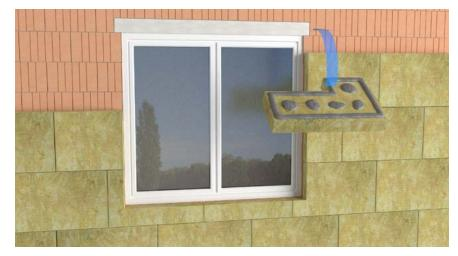
L shaped boards must be installed around all openings ensuring that no edge is smaller than 150mm and no piece of insulation smaller than 150mm throughout the installation.
