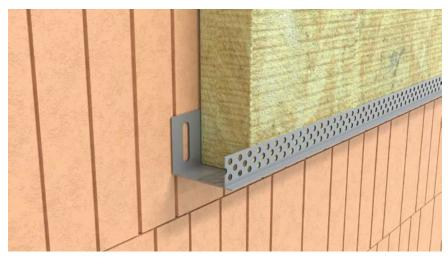
The first course of dual density mineral wool boards are placed into the SOLTHERM STATER TRACK.
