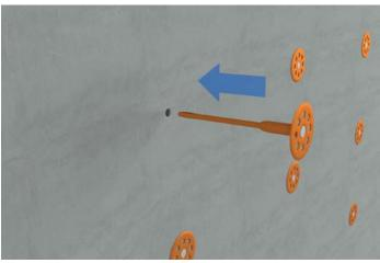
Place the fixing into the pre-drilled hole and push the fixing in until the head of the fixing is flush with the face of the base coat.
