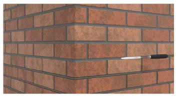
Once SOLTHERM KL pointing mortar has sufficiently picked up but remains ,green', point the mortar to the required method. Once complete, the walls are to brushed down with a soft brush at an approximate 45° angle, removing excess pointing mortar and cleaning the face of the brick slips.
