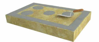
Repeat the contact layer application for 6-8 large dabs (80-100mm) to the centre of the board
