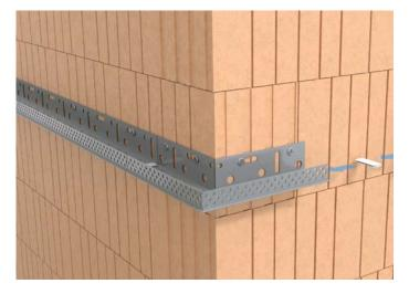
The SOLTHERM STARTER TRACK is installed at DPC level and at least 150mm above ground. The starter track is mechanically fixed at 300mm centres with specified fixing and approx. 50mm from the edge.
