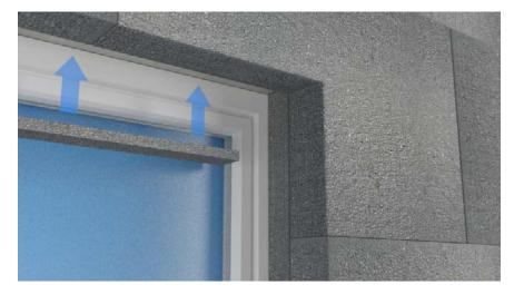
Where windows have recessed reveals and/or heads, oversail the insulation board beyond the existing to create a channel to set 20 mm or 30 mm thick EPS insulation strip in place within the reveal, adhesively fit as appropriate.
